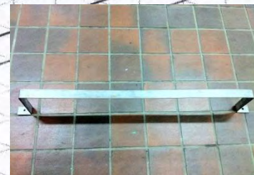
Bracket (Must follow contour of tank cover closely. Clearance between bracket & tank cover must not be more than 5 mm.)
